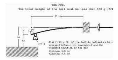
Figure 8. Foil dimensions and flexibility
