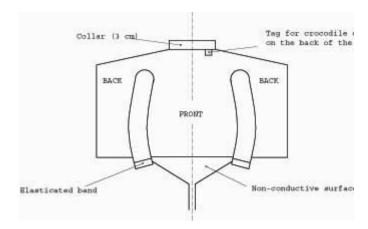
Figure 15. Electric saber conductive jacket
