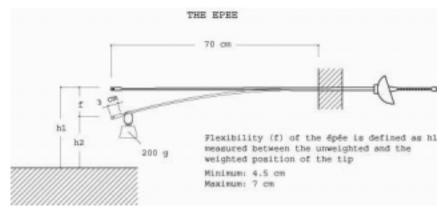
Figure 9. Epee dimensions and flexibility
