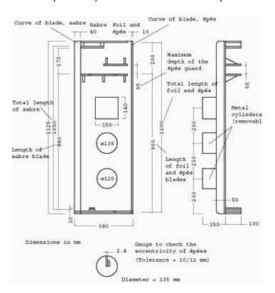
Figure 16. Gauge for checking weapons
