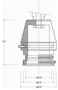
Figure A.3. Fixing device for test of cloth resistance to perforation
